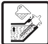
Indicates the required oil level in the crankcase
