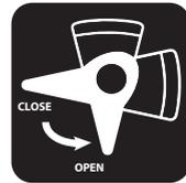
The "OPEN" position means open and the "CLOSE" position means closed
